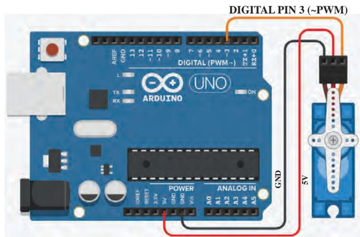
Fig 6.11 Smart Door System - Circuit
