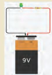
terminal of the LED is slightly longer than the cathode. To prevent excessive current flow and potential damage to the LED, a resistor must be connected in series with the LED circuit. The resistor's value depends on the maximum power the LED can handle and the voltage of the power source.
