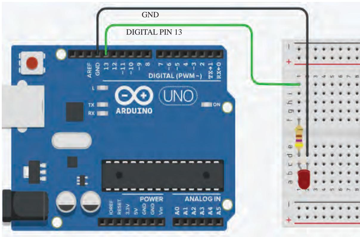
Fig 6.5 LED Circuit Connected in PIN 13 of Arduino
