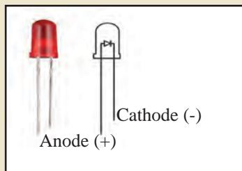
An LED is a two-terminal electronic device belonging to the diode category that conducts electricity in only one direction and emits energy in the form of light. Electricity will flow through the LED circuit only if its anode terminal is connected to the +ve of the battery and cathode to the -ve of the battery. Typically, the anode
