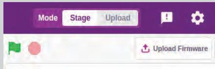
In this mode, the program prepared on the computer is completely uploaded to the memory of the Arduino microcontroller. Later, it does not require a computer to **run** the program. The Arduino only needs to be powered on.
