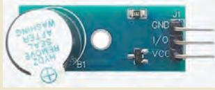
This is an electronic component used to produce a beep sound. It can be powered by connecting the VCC of the buzzer to the 5V of the Arduino and the GND of the buzzer to the GND of the Arduino. It produces sound when a LOW signal is given to the I/O PIN. The sound stops when a HIGH signal is received on the I/O PIN.
