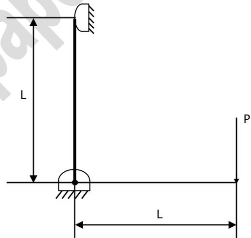
41. A uniform rigid rod of mass  $M$  and length  $L$  is hinged at one end as shown in the adjacent figure. A force  $P$  is applied at a distance of  $2L/3$  from the hinge so that the rod swings to the right. The reaction at the hinge is
