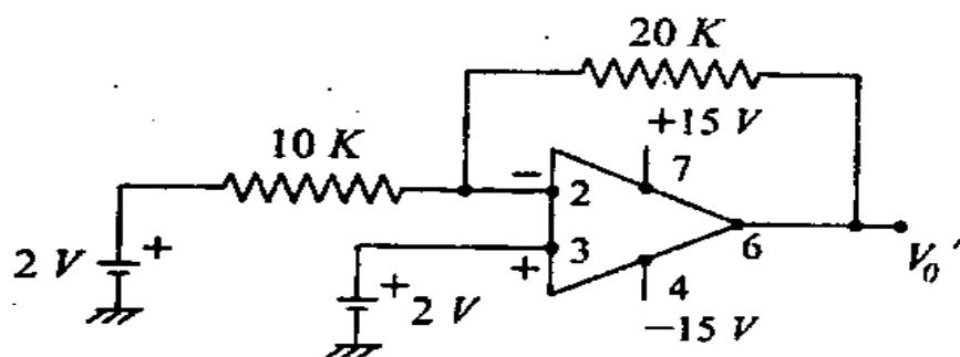
Identify the above op-amp circuit. Estimate the net output voltage  $V_o$ . 10
