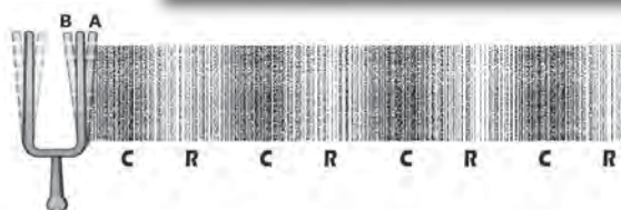
Pressure variations occurring in air when the tuning fork vibrates
