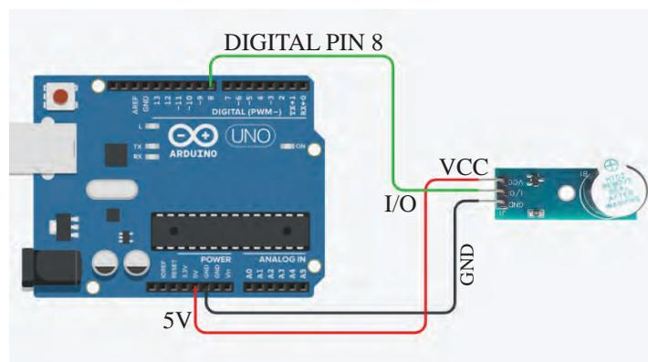
Fig 6.7 Circuit in which Buzzer is Connected
