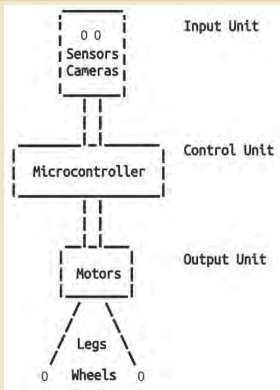
Robots use various types of sensors to perceive their surroundings. These sensors (input devices) gather information, which is then processed by microcontrollers or microprocessors. The choice of processor depends on the volume and complexity of the data to be processed. As the data requirements grow, the efficiency and number of processors are scaled accordingly. Based on the processed information, the robot's control unit manages the output devices.
