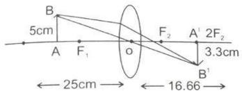
Since the value of the image is negative, indicates inverted (moving upside down) image the image is 3.3 cm in size at a distance of 16.66 cm behind the lens.
