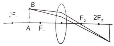
When the lower half of a convex lens is covered with black paper, the light rays from the object are refracted by the upper half of the lens, forming a reflection on the other side of the lens as shown in the figure.
