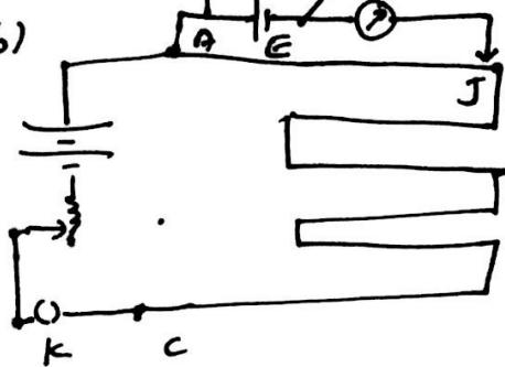
(c) potentiometer does not draw current from the cell, so it gives correct p.d. or emf. voltmeter only gives p.d.
