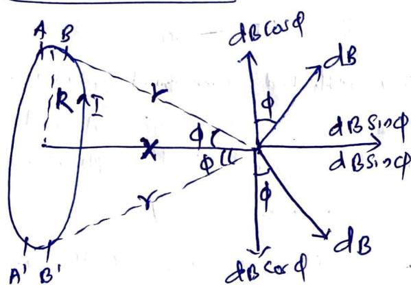
magnetic field due to current element AB,
