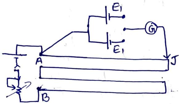
When  $E_1$  is connected to the circuit and let  $l_1$  be the balancing length, then,
