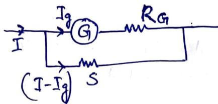
Galvanometer can be converted to ammeter by connecting a shunt resistance in parallel to galvanometer.
