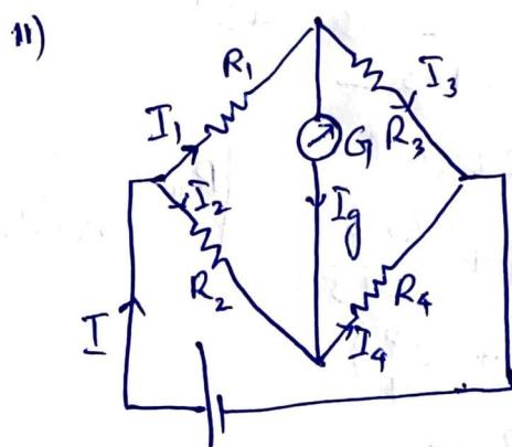
$$\text{when bridge is balanced } \frac{R_1}{R_2} = \frac{R_3}{R_4}$$
