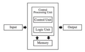
The mathematician John Von Neumann proposed a 'stored program computer' architecture which forms the basis of modern computers. His architecture consists of a CPU (Central Processing Unit) with ALU (Arithmetic and Logic Unit) and CU (Control Unit), I/O (Input/Output) unit and Memory unit.
