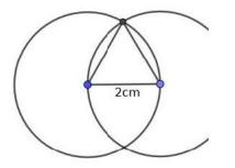
See the figure. One side of the triangle is given as 2 cm. What is the length of the other sides of the triangle?
