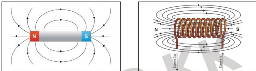
Tabulate the differences between the magnetic fields of a bar magnet and a solenoid
