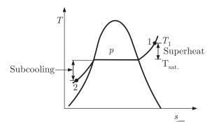
The pressure & temperature of compressed liquid may vary independently and a table of properties like the superheated vapor table could be arranged, to give the properties at any p & T.
