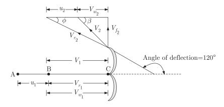
Given:  $u = u_1 = u_2 = 10 \text{ m/sec}$ ,  $V_1 = 25 \text{ m/sec}$ ,  $Q = 0.1 \text{ m}^3/\text{sec}$ Jet deflection angle= 120° C
