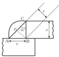
Given :  $l=60 \, \mathrm{mm} = 0.06 \, \mathrm{m}$ ,  $s=6 \, \mathrm{mm} = 0.006 \, \mathrm{m}$ ,  $P=15 \, \mathrm{kN} = 15 \times 10^3 \, \mathrm{N}$ Shear strength = 200 MPa
