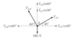
Resolve the  $T_{AB} \& T_{AC}$  in x & y direction (horizontal & vertical components)
