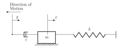
A small displacement gives to the system towards the left direction. Mass m is fixed, so only damper moves for both the variable x and y.
