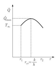
The rate of heat transfer from the insulated pipe to the surrounding air can be expressed as
