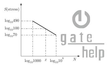
We know that in S-N curve the failure occurs at 10<sup>6</sup> cycles (at endurance strength) We have to make the S-N curve from the given data, on the scale of log<sub>10</sub>.
