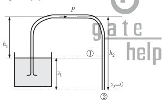
In a steady & ideal flow of incompressible fluid, the total energy at any point of the fluid is constant. So applying the Bernoulli's Equation at section (1) and (2)
