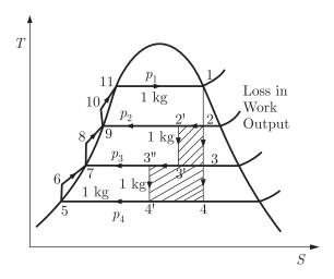
The thermal efficiency of a power plant cycle increases by increase the average temperature at which heat is transferred to the working fluid in the boiler or decrease the average temperature at which heat is rejected from the working fluid in the condenser. Heat is transferred to the working fluid with the help of the feed water heater.
