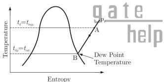
It is the temperature of air recorded by a thermometer, when the moisture (water vapour) present in it begins to condense.
