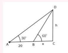
b) Triangle BCD is a  $30^{\circ} - 60^{\circ} - 90^{\circ}$  triangle .  $BC = x, h = \sqrt{3}x$ Triagle ACD is a  $30^{\circ} - 60^{\circ} - 90^{\circ}$  triangle .  $20 + x = \sqrt{3}h = \sqrt{3} \times \sqrt{3}x$  20 + x = 3x, 20 = 2x, x = 10 metre c) Height of the tree =  $\sqrt{3}x = 10\sqrt{3}$  metre d) Width of the river 10 metre
