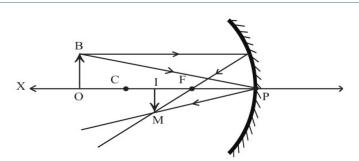
The figure shows the image formation when an object is placed beyond the centre of curvature C. The ray parallel and close to the principal axis has been considered. In the figure OBP and IMP are similar triangles according to the concept of similarity. Let s write down the ratio of corresponding sides of similar triangles.
