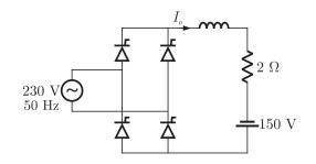
Assume that the load inductance is sufficient to ensure continuous and ripple free load current. The firing angle of the bridge for a load current of  $I_0 = 10$  A will be
