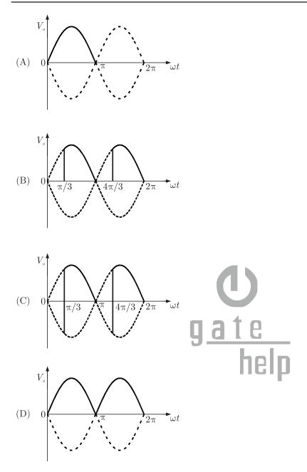
**Q.57** A 220 V 20 A, 1000 rpm, separately excited dc motor has an armature resistance of  $2.5 \Omega$ . The motor is controlled by a step down chopper with a frequency of 1 kHz. The input dc voltage to the chopper is 250 V. The duty cycle of the chopper for the motor to operate at a speed of 600 rpm delivering the rated torque will be
