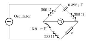
If the bridge is balanced for oscillator frequency f = 2 kHz, then the impedance Z will be (A)  $(260 + j0) \Omega$  (B)  $(0 + j200) \Omega$ (C)  $(260 - j200) \Omega$  (D)  $(260 + j200) \Omega$
