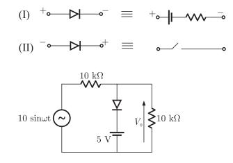
If such a diode is used in clipper circuit of figure given above, the output voltage  $V_0$  of the
