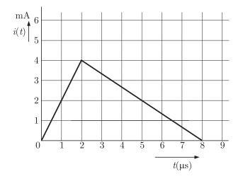
**Q.76** The charge stored in the capacitor at  $t = 5 \ \mu s$ , will be
