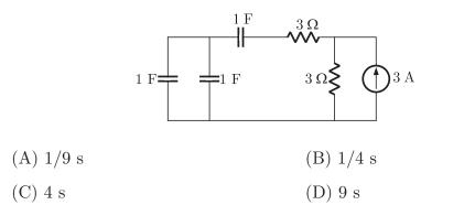
**Q.22** The resonant frequency for the given circuit will be
