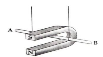
If the current passes from A to B, then in which direction the conductor will move?
