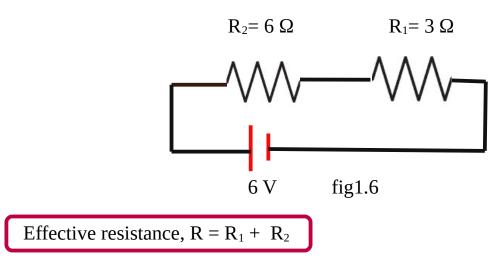
\* Effective resistance is the sum of the resistance of all the resistors when they are connected in series.
