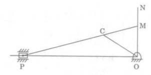
OCP is a slider-crank mechanism. OC = 10 cm is the crank. CP is the connecting rod = 22 cm; OP = 30 cm. ON is perpendicular to OP. PC extended meets ON at M. OM = 7.5 cm, CM = 8.0 cm. Crank runs at 10 rad/s. Find the velocity of the piston in cm/s.
