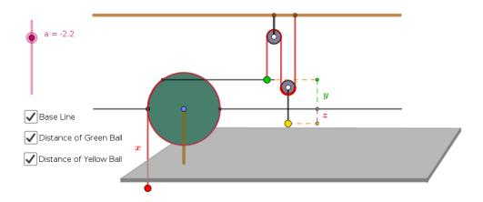
A rope is wound on a disc of radius 1 meter . A red ball is attached at the end of the rope. A green ball is attached to a point on the circumference of the disc by means of a rod which always remains horizontal. A yellow ball is attached to the green ball using two pulleys. We can wind/unwind the rope using the slider **a**. When  $\mathbf{a}=0$  all the balls lie on the base line, the horizontal line passing through the centre of the disc.
