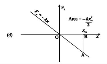
We have according to Hooke's law; the restoring force is proportional to the displacement of the spring. We can express Hooke's law as,
