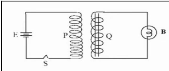
when the switch S is turned on, the bulb suddenly glows and turns off
