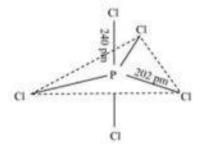
Three equatorial bonds are equivalent while the two axial bonds are longer than equatorial
