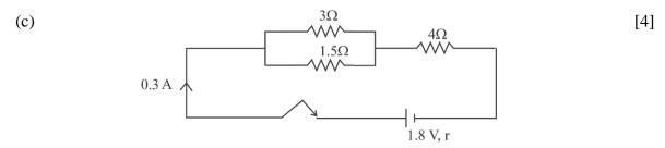
The diagram above shows three resistors connected across a cell of e.m.f.
