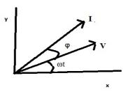
The diagram representing alternating voltage and current (phasors) as the rotating vectors along with the phase angle between them is called phasor diagram.
