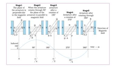
• In most generators, the coils are held stationary and it is the electromagnets which are rotated.
