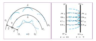
Huygens argued that the amplitude of the secondary wavelets is maximum in the forward direction and zero in the backward direction
