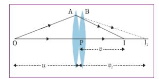
For the first lens, object is at O and image is at I<sub>1</sub>.
