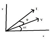
The diagram representing alternating voltage and current (phasors) as the rotating vectors along with the phase angle between them is called phasor diagram.
