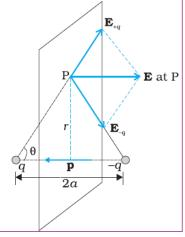
The magnitudes of the electric fields due to the two charges +q and -q are equal and given by
