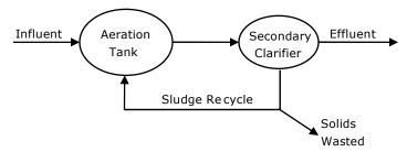
50. The food-to-biomass (F/M) ratio (in kg BOD per kg biomass per day) for the aeration tank is
