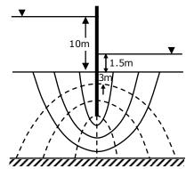
48. The seepage loss (in m³ per day per unit length of the wall) of water is
