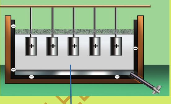
Molten Cryolite and Alumina
