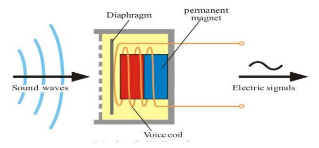
Which are the main parts of a moving coil microphone?
