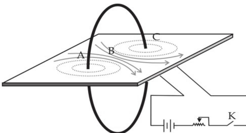
After passing current find the direction of magnetic field at C (shown in diagram) using a compass needle and mark it on the cardboard.
