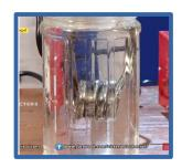
• Why the blade fell down, when switch is turned off? **Electromagnet is a temporary magnet.** It has magnetic property only when electricity is passes through it.
