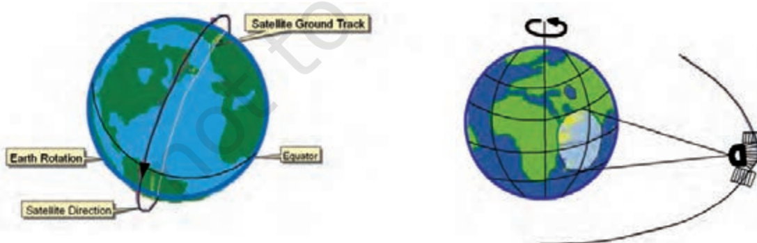
Figure 7.6 Orbit of Sun Synchronous (Left) and Geostationary (Right) Satellites
