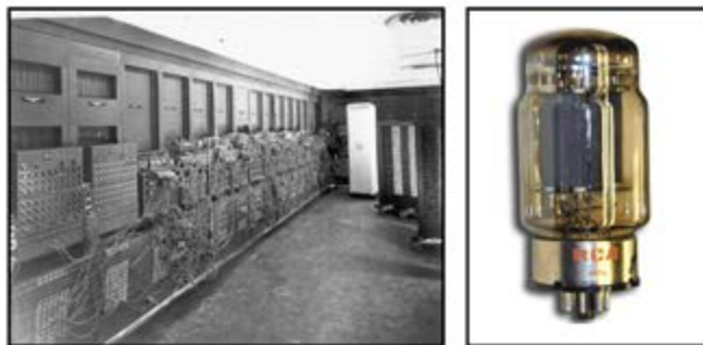
Fig. 1.13 : ENIAC and Vacuum tube
