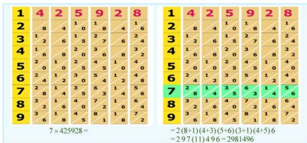
Fig. 1.4 : Multiplication using Napier's Bones
