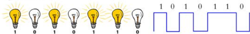
Fig. 2.2 : Digital representation of ON and OFF
