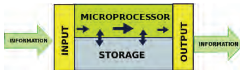
Illustration 10.1 Working of CPU
