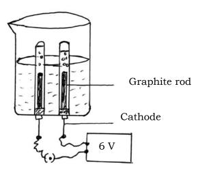
( Cathode can be labelled by connecting graphite rod to the negative terminal of the battery )  $1+\frac{1}{2}+\frac{1}{2}$
