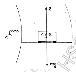
The forces acting on the car are: (i) the weight of the car, **mg**
