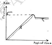
When we push or pull a body the static friction develops in the opposite direction. If we increase the external force, more and more static friction is developed. But the static friction has a maximum value called the limiting friction. If we apply more force than the limiting friction, the body will move. When the body once starts motion, the friction slightly decreases and thereafter it has a constant value called kinetic friction.
