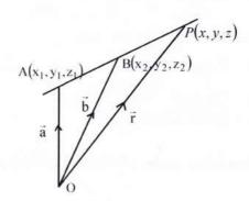
Cartesian equation of a line passing through two points  $A(x_1, y_1, z_1)$  and  $B(x_2, y_2, z_2)$  is  $\frac{x - x_1}{x_2 - x_1} = \frac{y - y_1}{y_2 - y_1} = \frac{z - z_1}{z_2 - z_1}$
