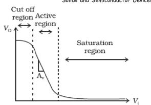
decreases linearly till its value becomes less than 1V. On further increasing  $V_i$ , the change of  $V_0$  with  $V_i$  becomes non - linear and the transistor inters into saturation state. The variation of  $V_0$  with  $V_i$  is shown in fig. This is called transfer characteristics.
