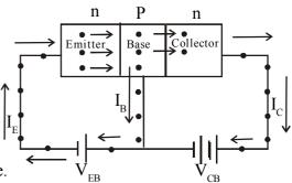
As a result, the collector collects the electrons. This produces a current in the collector, called collector current ( $I_c$ ). At the same time, the holes in the base region combines with the electrons from the emitter and a small current will flow in the emitter base circuit. This current is called base current ( $I_p$ ).
