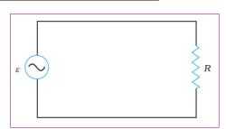
• The ac voltage applied to the resistor is
