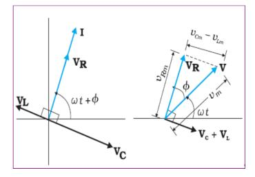
The length of these phasors V<sub>R</sub>, V<sub>C</sub> and V<sub>L</sub> are:
