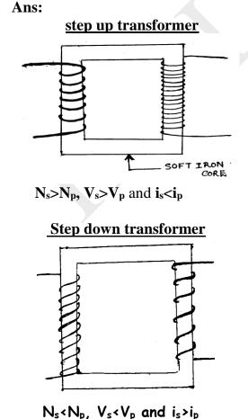
Let  $N_p$  and  $N_s$  be the number of turns in the primary and secondary of the transformer. The voltage induced in the secondary, when **AC** flows through the primary is given by
