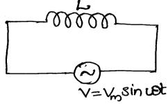
Consider an AC voltage  $v = v_m \sin \omega t$  applied to an inductor (L)  $V = v_m \sin \omega t \dots (1)$
