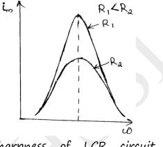
Sharpness of LCR circuit is defined as " the ratio of resonant frequency to the band width"
