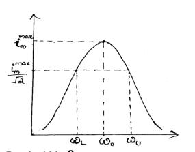
Band width,  $\beta = \omega_U - \omega_L$  $\omega_L$  is the Lower cut off frequency and  $\omega_U$  is the Upper cut off frequency Note :- The resonance curve is sharp if the band width is small.
