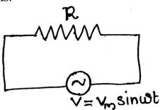
Consider an a.c. voltage  $v = v_m \sin \omega t$  applied to a resistor R.  $v = v_m \sin \omega t \dots (1)$ Dividing equation (1) by R
