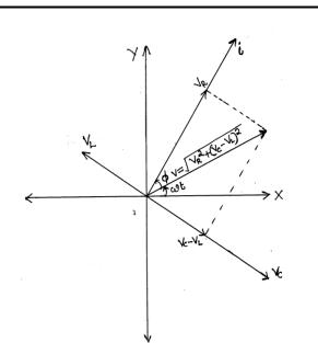
Consider an a.c. voltage  $v = v_m \sin \omega t$  applied to a series circuit containing an **inductor** (L), **capacitor** (C) and a **resistor** (R).
