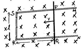
The straight conductor PQ is moved towards the left with a constant velocity v perpendicular to the uniform magnetic field B.
