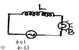
L is called **self inductance** of the coil or coefficient of self induction According to Lenz's law.
