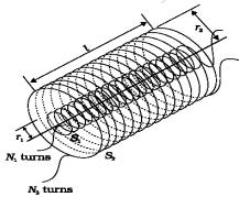
Let a current  $I_2$  flows through  $S_2$ . Then the magnetic flux linked with  $S_1$  is  $\Phi_1=M_{12}$   $I_2$  ----- (1)
