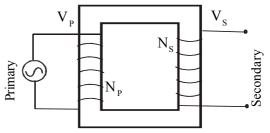
$\therefore \frac{E_P}{N_P} = \frac{E_S}{N_S} \qquad or \quad \frac{E_P}{E_S} = \frac{N_P}{N_S} = K \text{ where K is called Transformer ratio or turns ratio of}$
