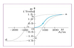
The closed curve abcdea which represents a cycle of magnetisation of a ferromagnetic sample is called its hysterisis loop.
