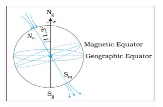
A vertical plane passing through the magnetic axis of a freely suspended magnet is called the magnetic meridian.
