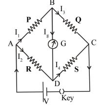
When no current flows through the galvanometer, the bridge
