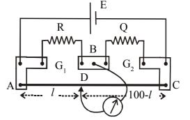
be balanced. The position of the jockey where galvanometer shows no deflection is called *null point*.
