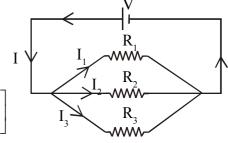
Now if the three resistors are replaced by a single resistor of resistance R, then  $I = \frac{V}{R}$
