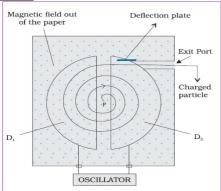
The whole device is in high vacuum so that air molecules do not collide with charged particles.
