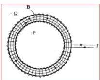
Toroid is a hollow circular ring on which a large number of turns of a wire are closely wound.
