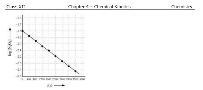
(iv) The given reaction is of the first order as the plot,  $\log[N_2O_5]_{v/s} t$ , is a straight line. Therefore, the rate law of the reaction is
