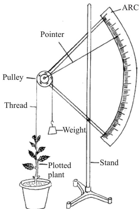
**Fig. 20.3** Auxanometer
