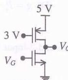
Q.57 For small increase in  $V_G$  beyond 1 V, which of the following gives the correct description of the region of operation of each MOSFET ?
