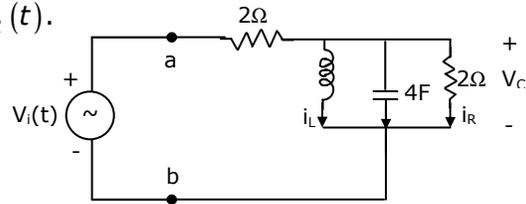
5. For the circuit in Fig.P5, write the state equations using  $v_c$  and  $i_L$  as state variables.
