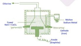
A graphite block is the anode while steel is made the cathode. Metallic Ca and Na are formed at the cathode. Molten Na is supported by dipping in kerosene.
